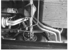
Install the passenger side over axle tailpipe #C onto muffler at least 1-1/2" to 2" using clamp #F to attach tailpipe. Do not tighten. Install Driver side over axle tailpipe #D onto Muffler at least 1-1/2" to 2" using hanger #H to attach tailpipe. Insert into rubber grommet.
